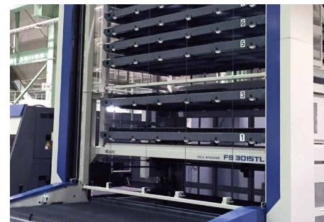
Loading Laser Pallets on the shelf
