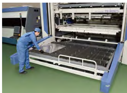
Placing the material by handing
